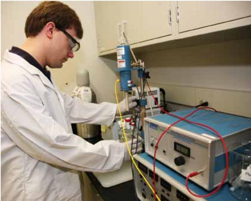
**Figure 3.** Using a Rotating Ring Disk Electrode, Adam Lemke conducts leading-edge research at CNSE's Center for Sustainable Ecosystem Nanotechnologies.
