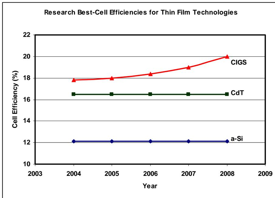
Figure 1 shows the best research cell conversion efficiencies for the three technologies, verified by NREL.<sup>5</sup> Cell efficiencies have not improved for CdTe and a-Si technologies since 2004 whereas they have consistently increased each year for CIGS. The cell efficiency of CIGS at the end of 2008 was 20%, ahead of the 16% achieved by CdTe.
