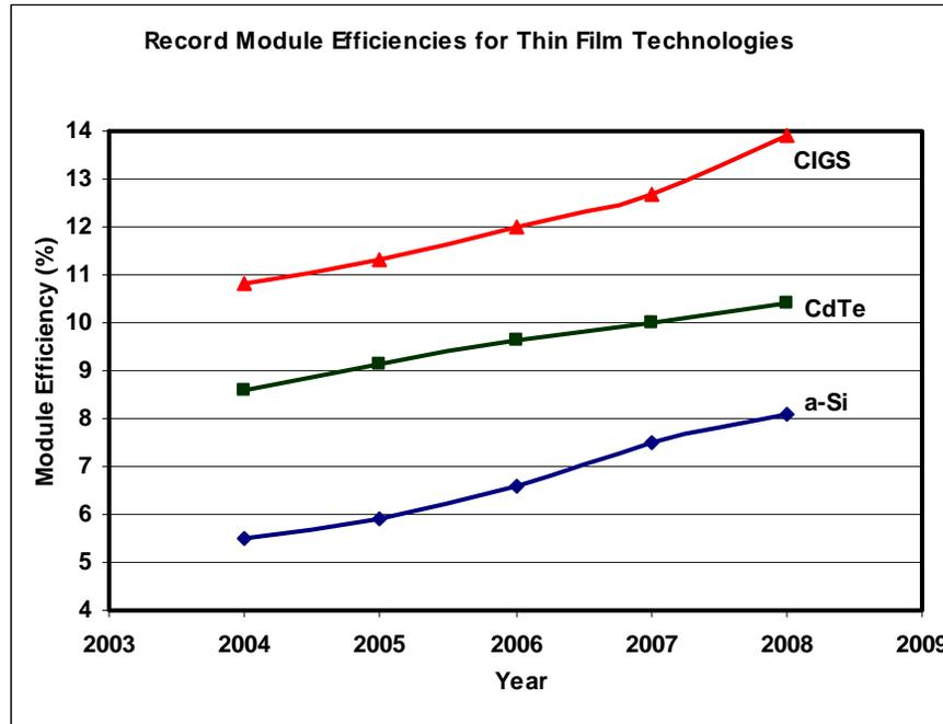
Figure 2 shows the module efficiencies for the three technologies.<sup>6</sup> Note that CIGS has consistently had higher module efficiency than both a-Si and CdTe for all years in 2004-2008.
